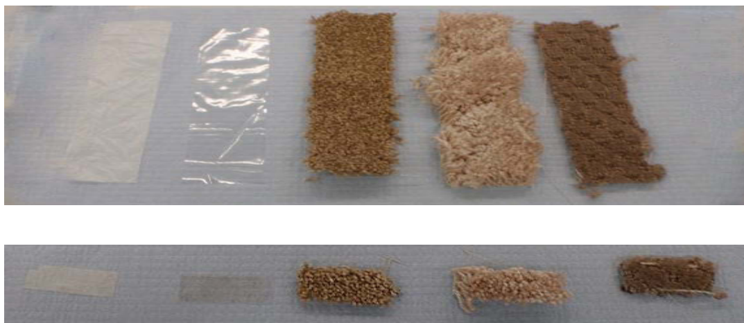
Figure 2.2 Samples before (top) and after burial (bottom)
