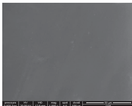
Figure 4.5 SEM micrograph of PVC after burial in the dry environment for 3 months
