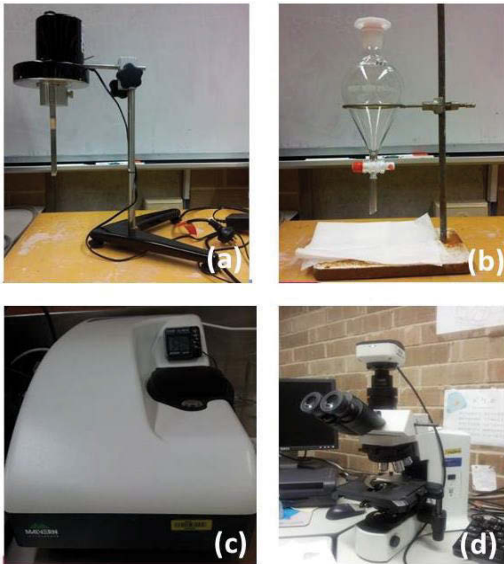
Fig. 3.7. The instruments for analysis of sludge samples: a) Brookfield Viscometer M/00-151-E0808 for sludge viscosity; b) Separatory funnel for RH; c) Zetasizer Nano ZS for zeta potential; d) Olympus System Microscope Model BX41 for obtaining images of sludge flocs
