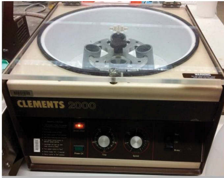
Fig. 3.5. Photo of centrifuge (Clements 2000)
