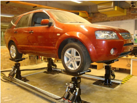
Figure 7. 2: Four poster suspension test rig
