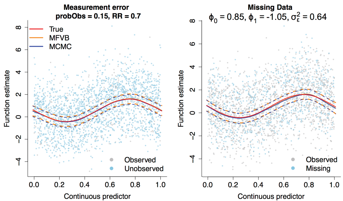
Figure 4.5: Approximate posterior means of the penalised regression functions and corresponding pointwise 95% credible sets obtained via MFVB approximation (orange curves) and MCMC (blue curves) for a single replication of the simulation study described in the text. The red curves represent the true mean functions. The grey circles represent the observed data and the sky blue circles represent the unobserved or missing data.
