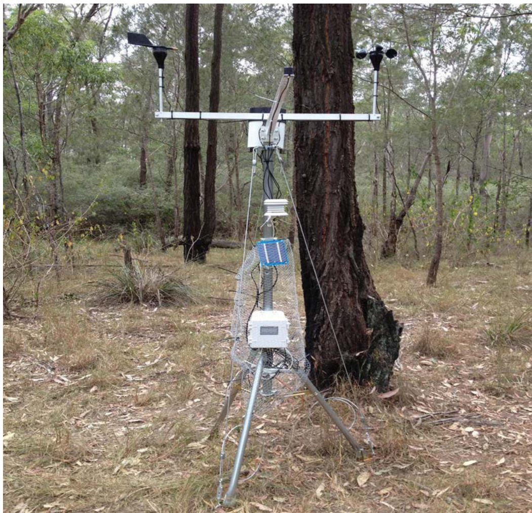
Figure 2-4: Weather station set-up, recording rainfall, temperature, relative humidity, wind speed and direction and solar radiation.
