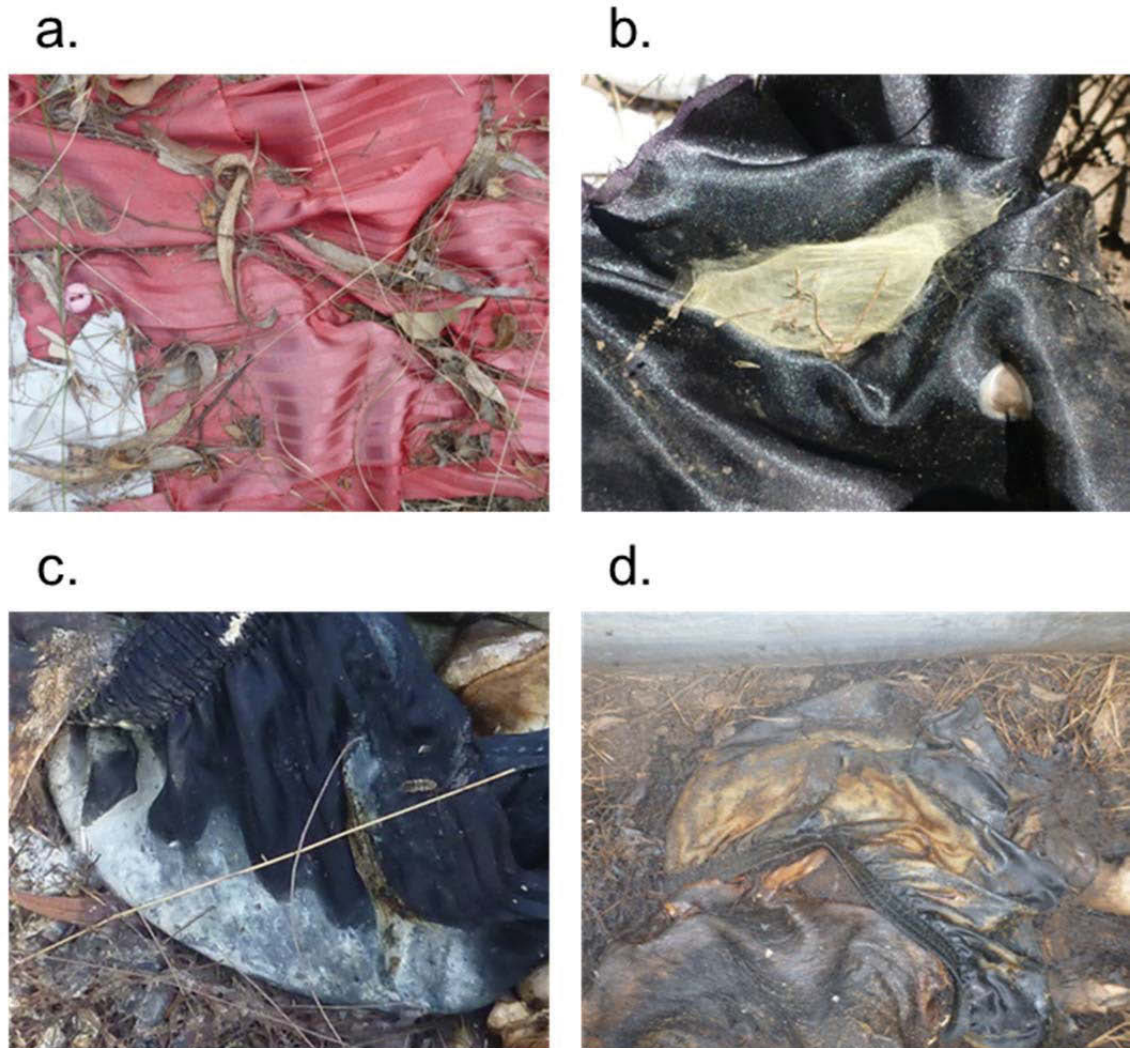
Figure 3-10: Visual damage to the polyester briefs from a) a control site after 365 days; b) a control site showing the presence of insect activity on day 247; c) an experimental site after 24 days with sections of white deposits; and d) an experimental site after 31 days with visible orange/brown staining.
