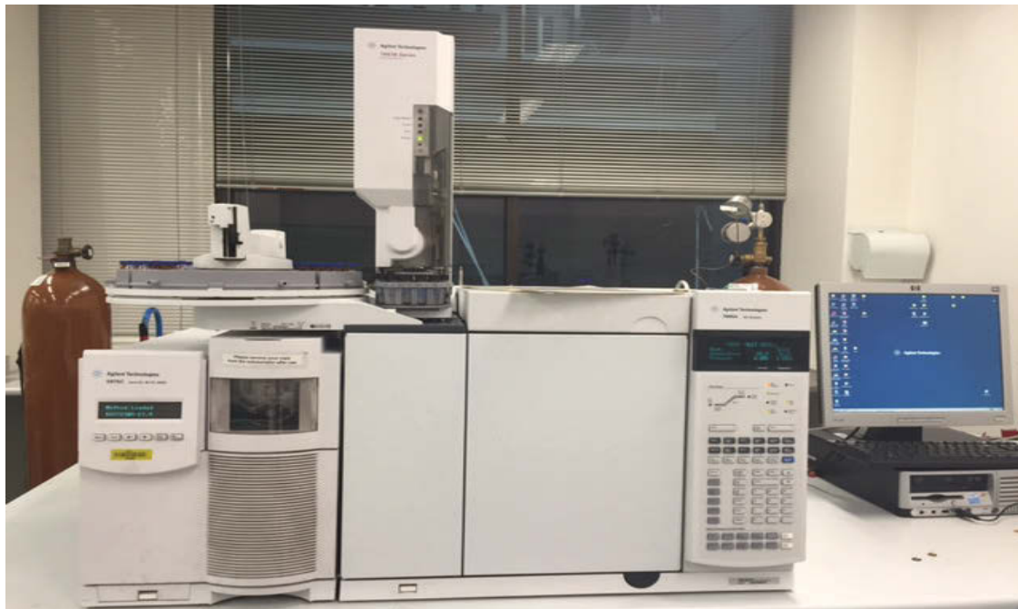
Figure 2-6: Agilent 7890A gas chromatograph coupled to an Agilent 5975C mass selective detector.
