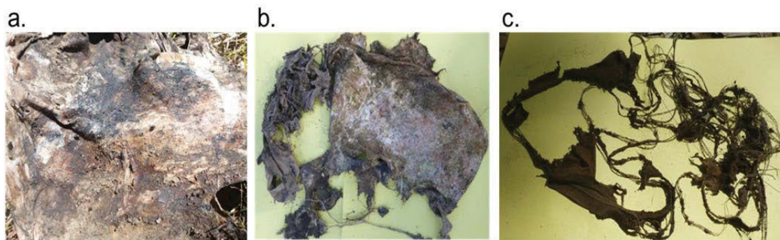
Figure 7-5: Textile damage observed with cotton samples from the pig graves after a) 9 months, b) 18 months and c) 24 months.
