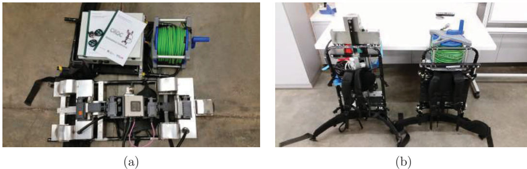
FIGURE 5.18: Backpacks used to deploy robot at site. (a) Two backpacks are shown, top, containing control unit and tether, bottom, containing robot. (b) Each backpack is 18kg and uses ergonomic straps for the inspectors to carry.
