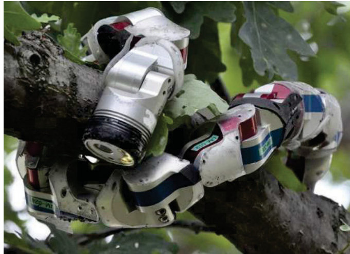
FIGURE 2.3: Snake type robot climbing a tree branch through means of grasping and bracing. [46]
