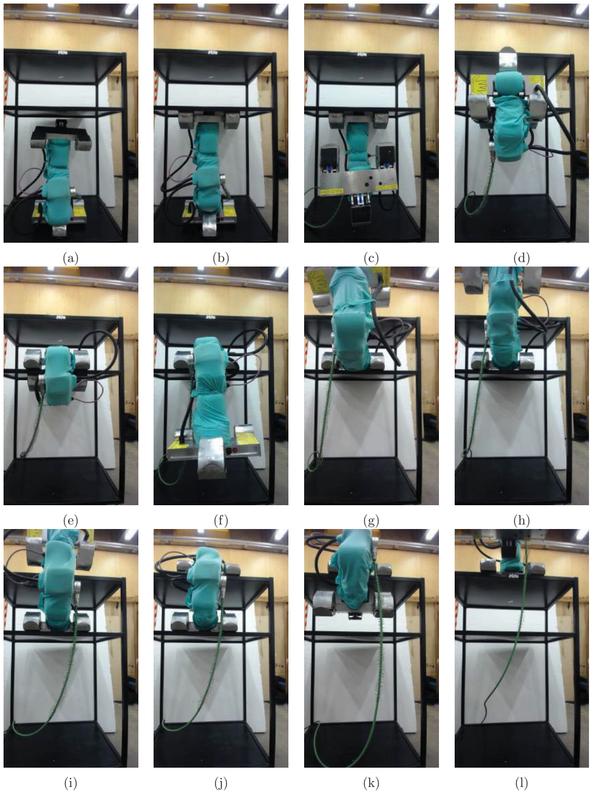
FIGURE 5.17: Demonstration of the inchworm-inspired climbing robot performing 180^\circ plane transition and discontinuity transition.
