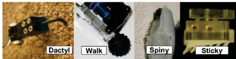
FIGURE 2.8: Four different feet variants used by the RiSE climbing robot. [83]
