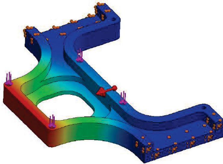
FIGURE 5.5: Finite Element Analysis of links. Figure shows the primary bracket used on joints 1 and 7. The bracket provides additional reach ability for the 180^\circ plane transition, and is subject to the greatest load torque. FEA was used to reduce weight and minimise deflections under load.
