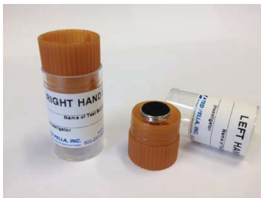
Figure 1-1: Gunshot residue collection kit with double-sided adhesive on aluminium stubs
