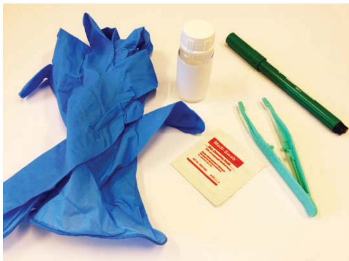
Figure 5-1: Swabbing kit used for the collection of gunshot residues by medi wipes. The kit includes a pair of gloves, plastic tweezers, a scintillation vial, Kendall™ alcohol swab, and pen.
