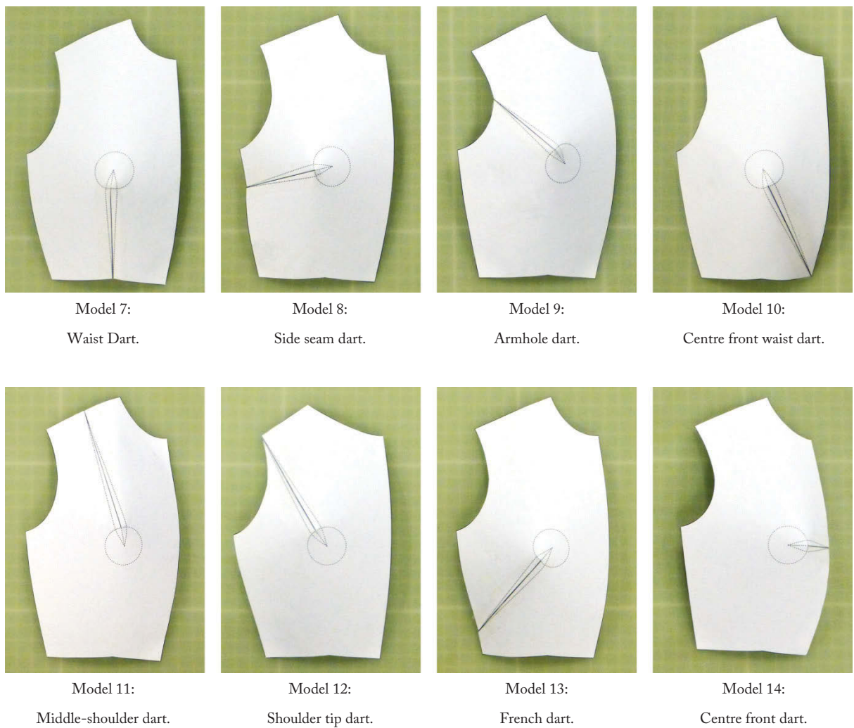
Figure 6: A detailed view of patterns with different dart locations created using bust point manipulation.
