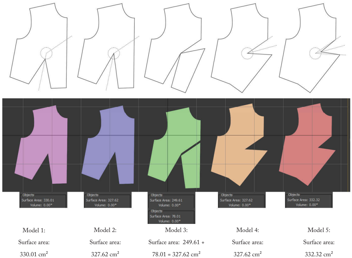
Figure 4: Patterns digitized in 3DS Max (Autodesk 2012). The surface area of model 1 is different from the surface area of model 5.
