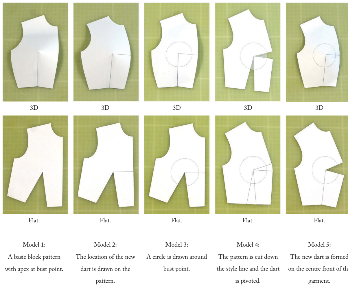
Figure 1: A new dart line is drawn on the basic block pattern and the dart is moved at bust point to the new location.
