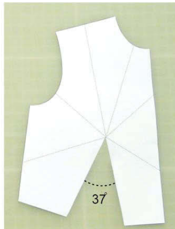
Model 8: Draw six straight style lines on the pattern. The dart angle measures 37°.
