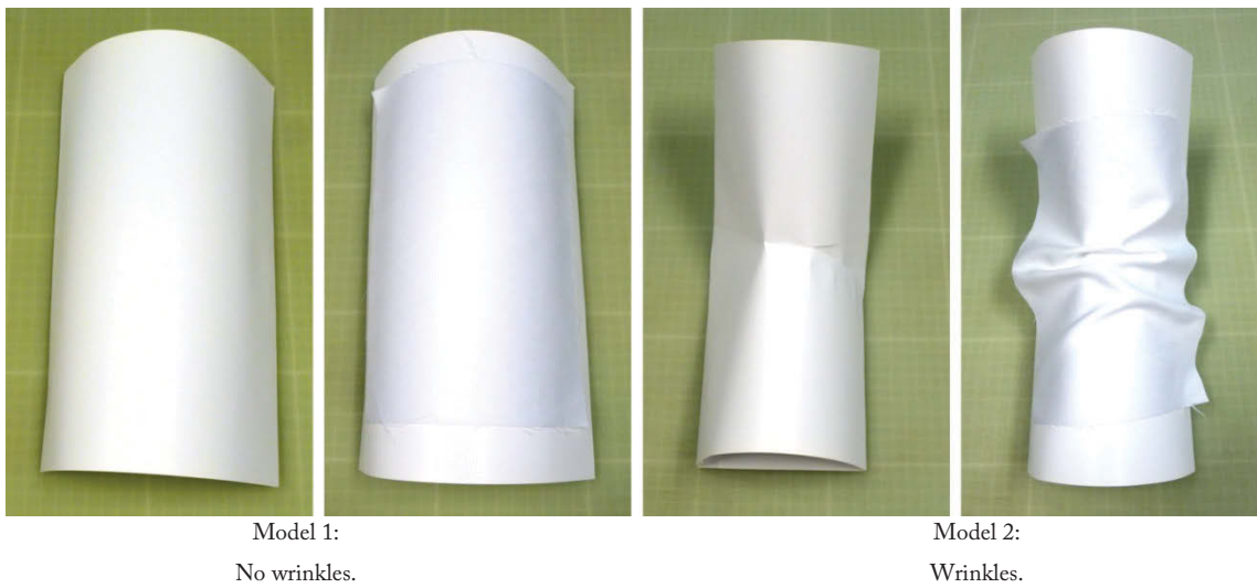
Figure 3: A physical model of Figure 2 demonstrating wrinkling on a hyperbolic surface.
