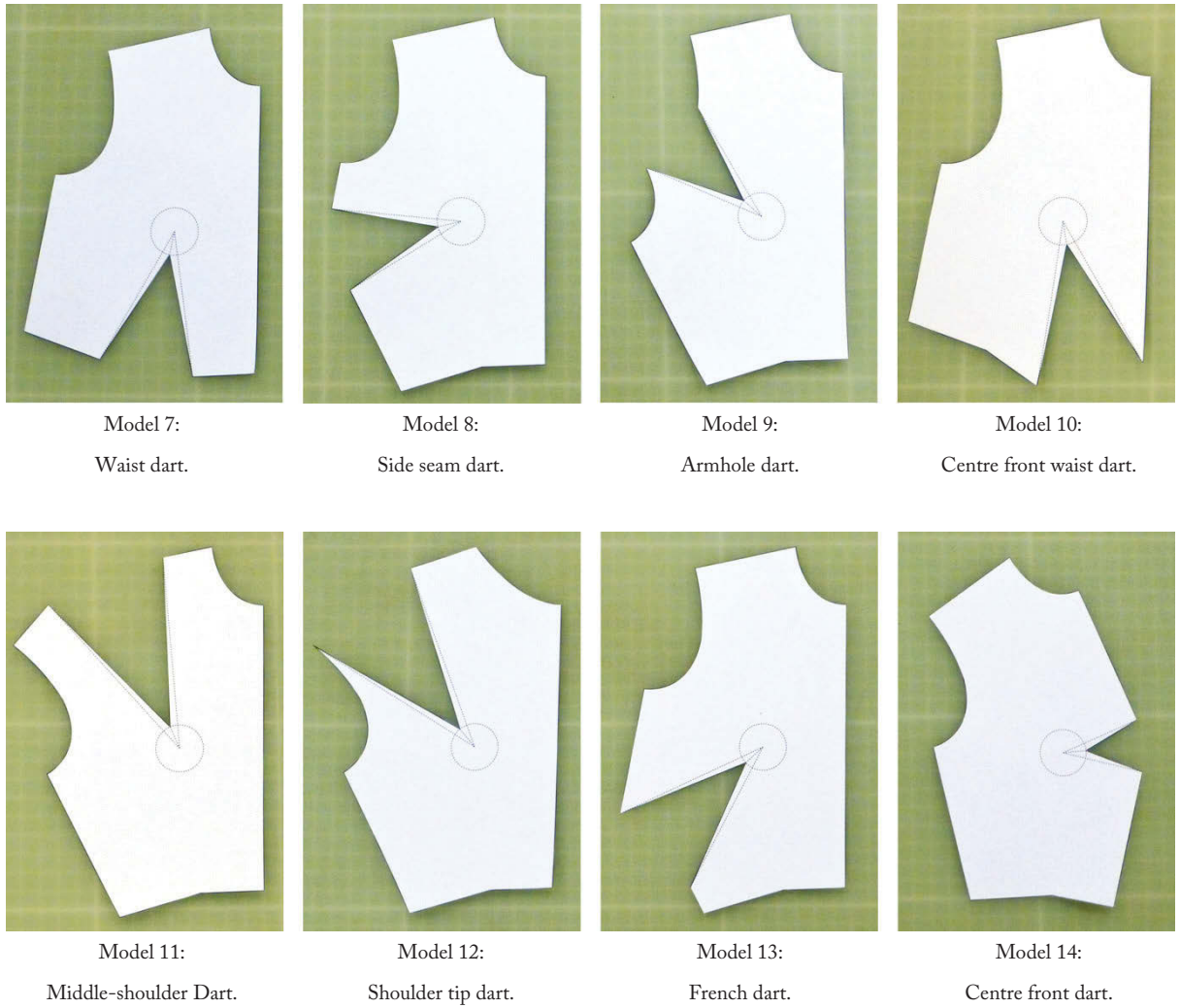
Figure 7: A detailed view of the flat patterns with different dart locations created using bust point manipulation.
