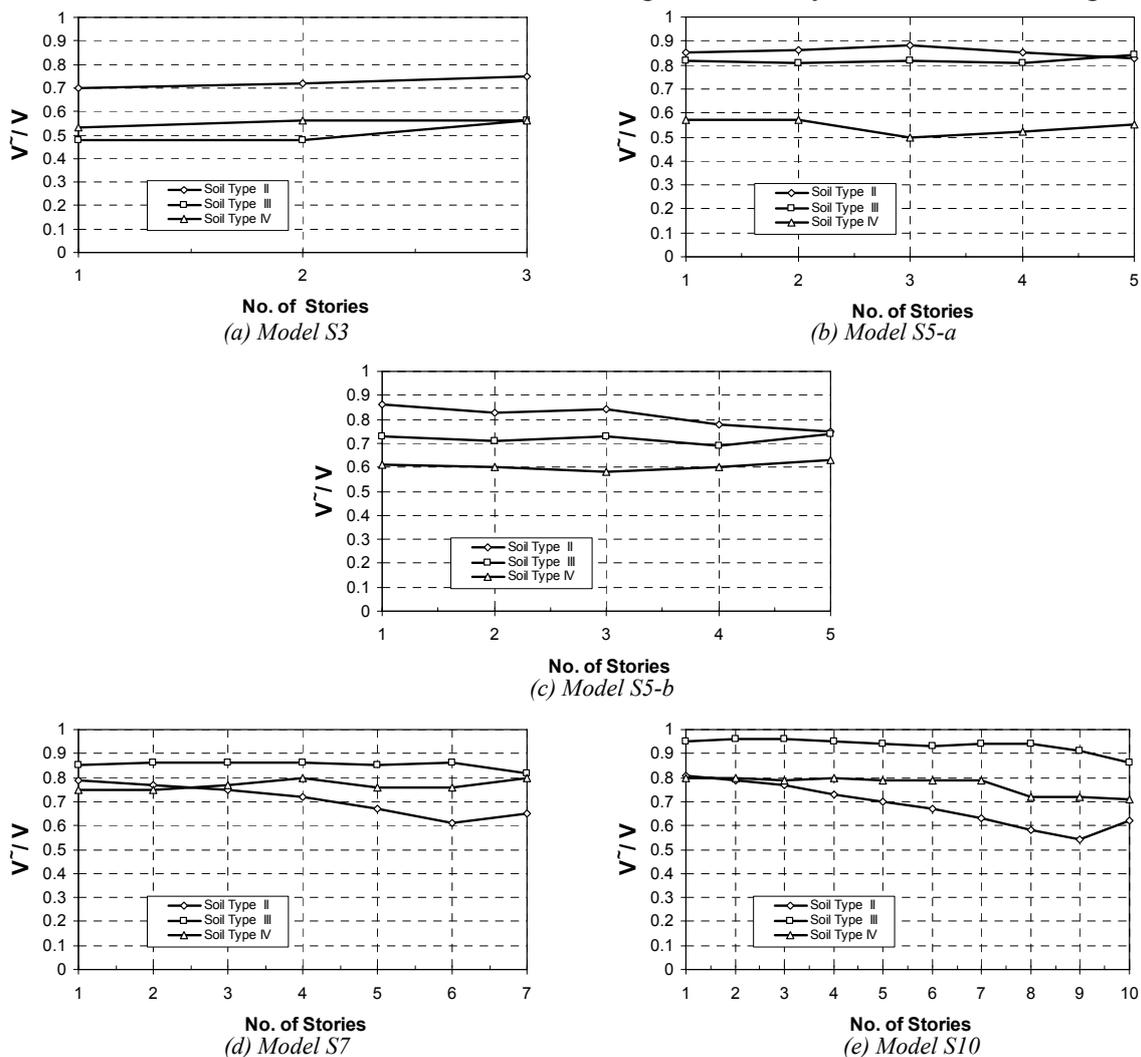
Figure 5 Average Ratio of story shear of flexible base to fixed-base on soil types II, III and IV
