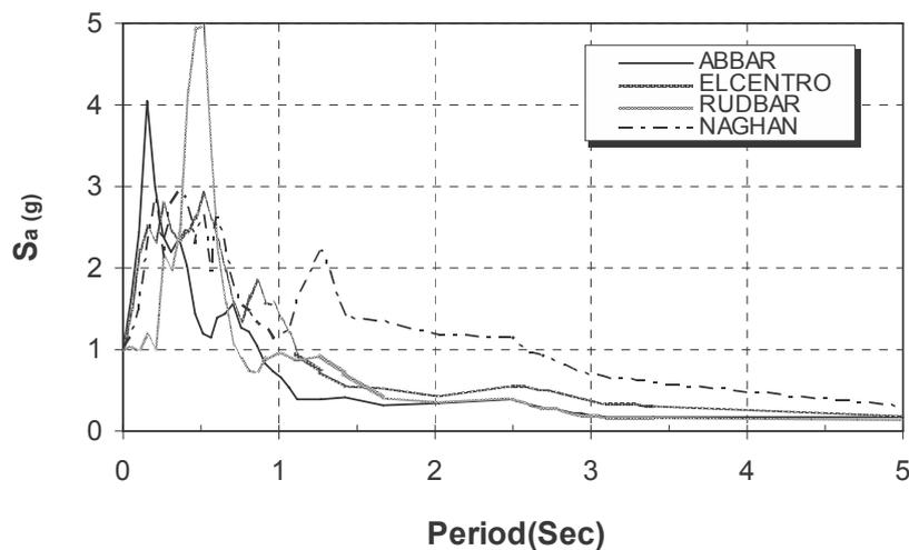
Figure 2 Respond Spectra of used acceleration records
