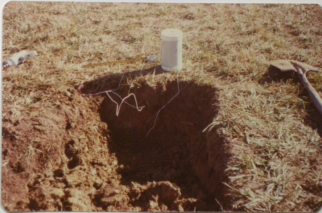
Photo 3-13 Installation of Thermocouples - Station No 1
