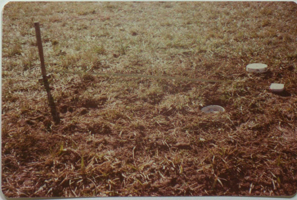
Photo 3-14 Completed Installation of Thermocouples Station No 1
