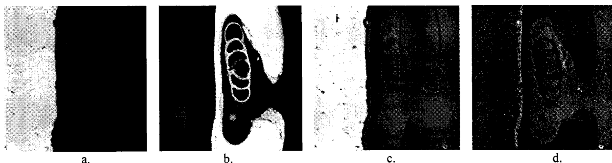
Figure 1: A barnacle attached to an aluminium plate which has been set in a resin, sectioned and polished. a) RIOM for aluminium, b) RIOM for calcium c) RIOM for chlorine and d) QXRM for chlorine. Region (i) is the aluminium plate with <0.02 wt% Cl (less than the EDS detection limit), region (ii) is the barnacle with ~0.03 wt% Cl and region (iii) is the resin with ~1.3 wt% Cl (HWOFF=260um).
