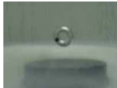
Fig. 2. Levitation of a free spin PM on a HTS disk.
