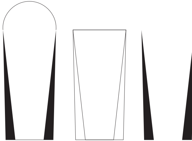
FIGURE 2.8: Schematic of sheath volume calculation as approximated by the difference between two inverted truncated cones. Left is a profile view of the pillar, cap, core and sheath. Middle is the two inverted truncated cones that define the inside and outside of the sheath. Right is the volume from the difference, the sheath volume.
