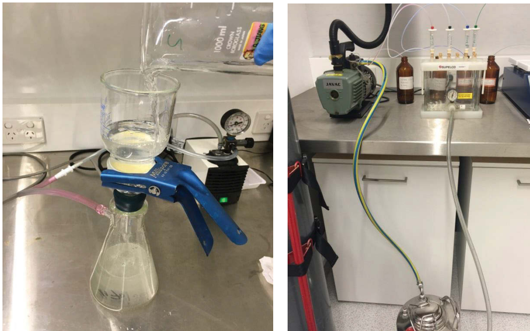
Figure 3.8 Procedure used for SPE for analysing micropollutants
