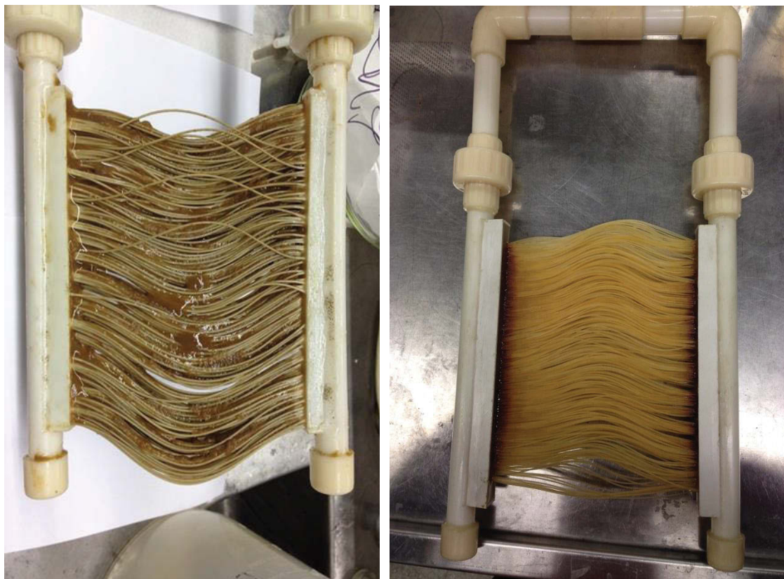
Figure 6.21 Comparison of fouled membrane and after physical and chemical cleaning
