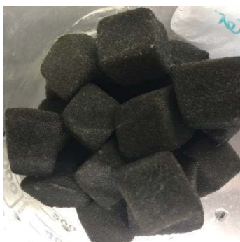
Figure 3.1 The attached-growth carriers (sponge cubes) used in this study
