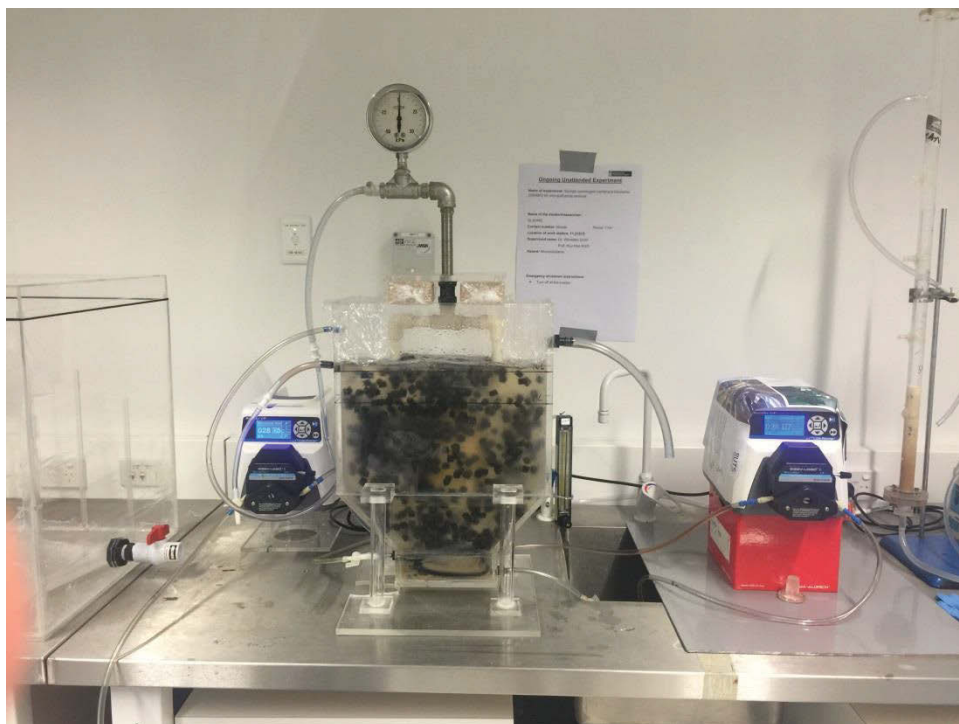
Figure 3.4 On-site photo of the SSMBR system
