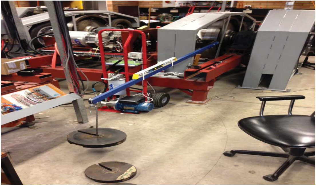
Figure 5-6: Torque sensor calibration (a)
