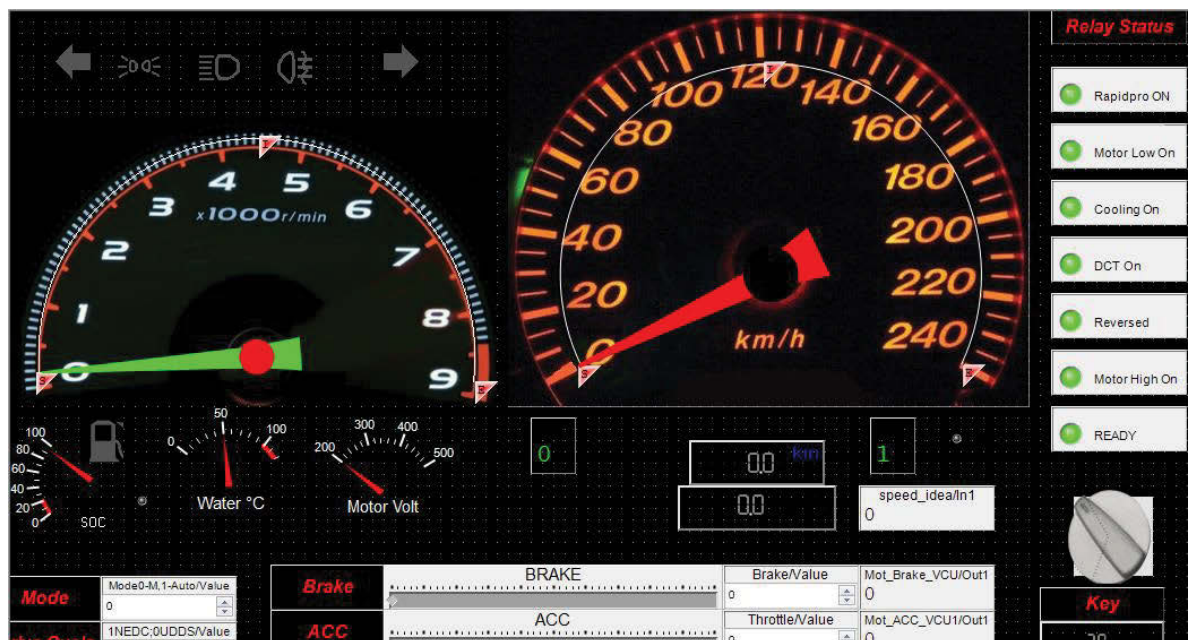
Figure 5-13: PC display panel for data acquiring, variables changing in ControDesk®
