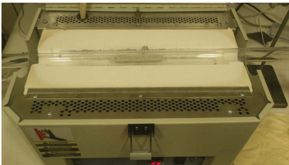
Figure 3.1. Photograph of the annealing tube furnace.
