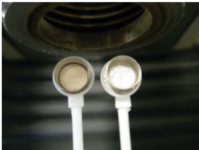
Figure 7-1. Photographic image of the sample holder configuration of a SDT 2960 with simultaneous TGA-DSC. The sample under analysis is in the left crucible, the right crucible is a reference used for DSC measurements
