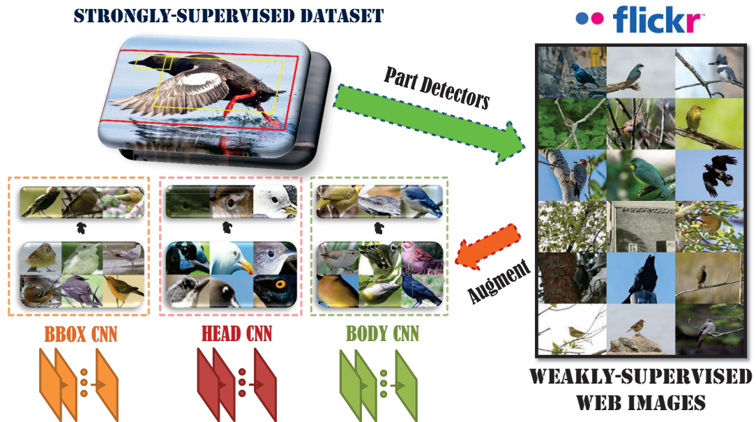
Figure 6.1: Illustration of the proposed semi-supervised method via web data. A strongly supervised dataset is introduced to “teach” web images how to learn properly.
