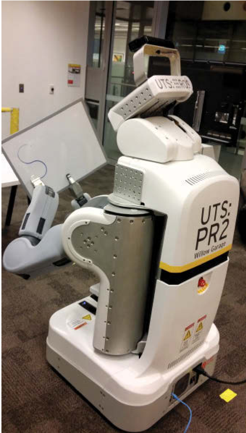
Figure 6.18: PR2 robot writing on the board using MAGIKS off-line IK engine in TP scenario
