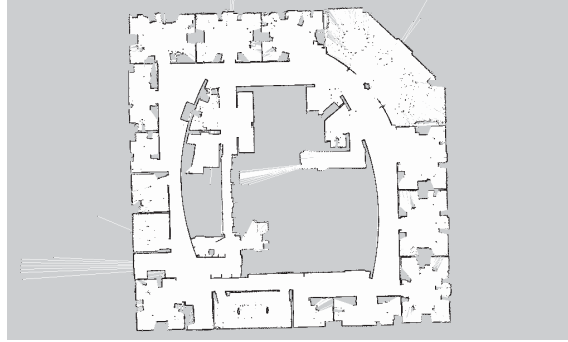
FIGURE 4.1: An occupancy grid map of the Intel Research Laboratories, Seattle, USA generated using GMapping.
