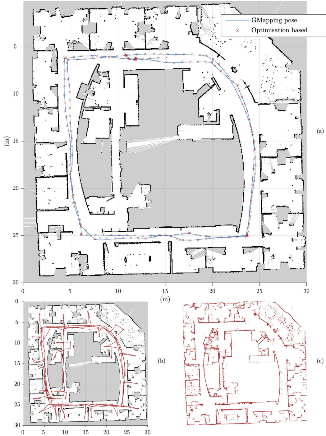
FIGURE 3.8: Trajectory of the robot in the Dataset 2. (a) GMapping poses and results obtained from the optimisation based localisation strategy. (b) Complete trajectory. (c) Projection of the laser scan from the estimated pose.
