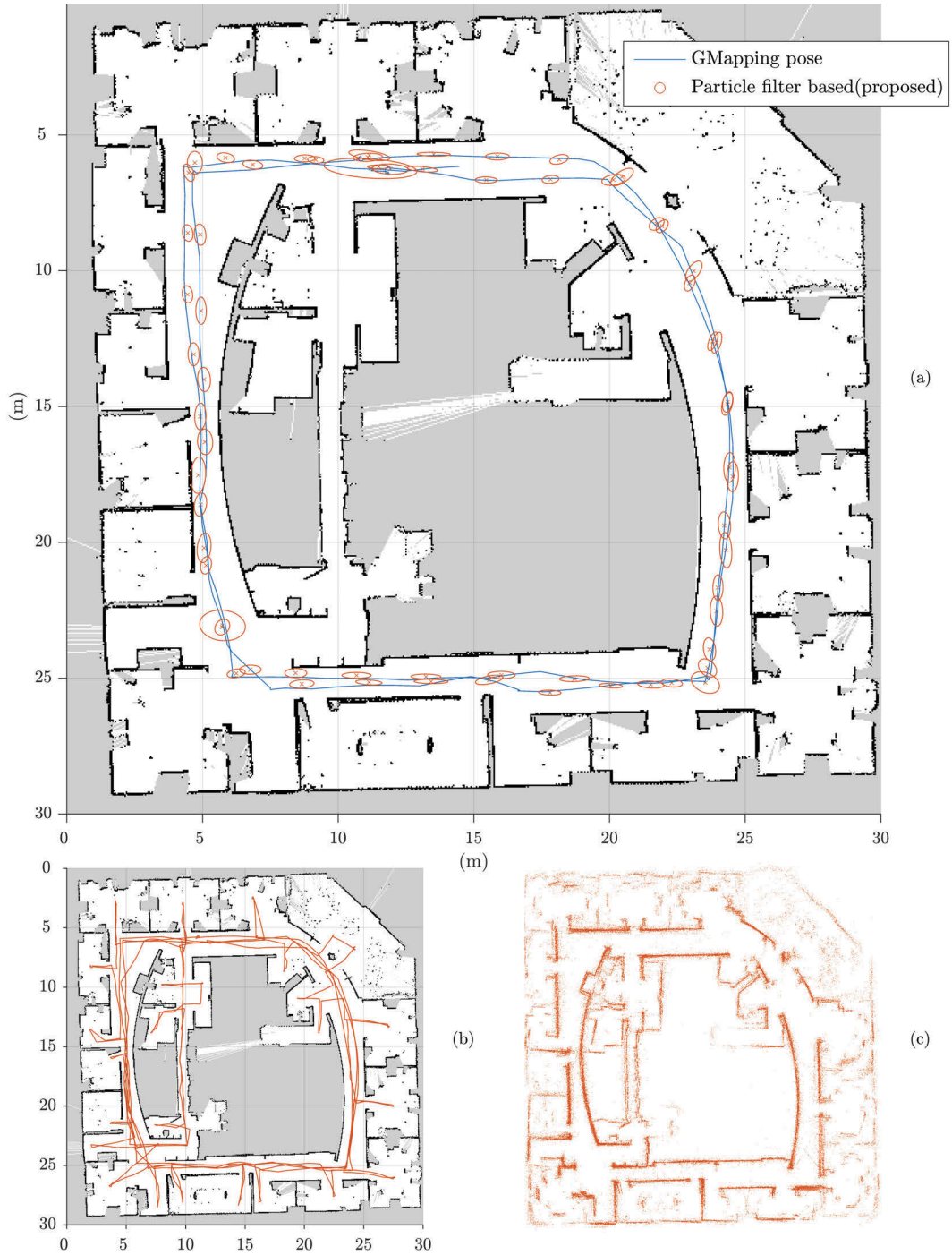
FIGURE 3.9: Trajectory of the robot in the Dataset 2. (a) GMapping poses and results obtained from the particle filter localisation algorithm, with uncertainty ellipses. (b) Complete trajectory. (c) Laser projection from the localised pose.
