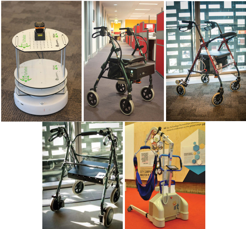
FIGURE 1.1: The robots we used to collect real-time data for experiments presented in this thesis. In sequential order: Turtlebot - modified, Walker revision 1, Walker revision 2, Motorised Walker, Smart Hoist
