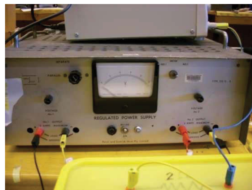
Fig. 3.36 Power supply used for current sensor board from NI
