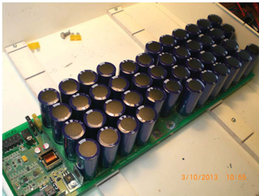
Fig. 3.86 A single supercapacitor module
