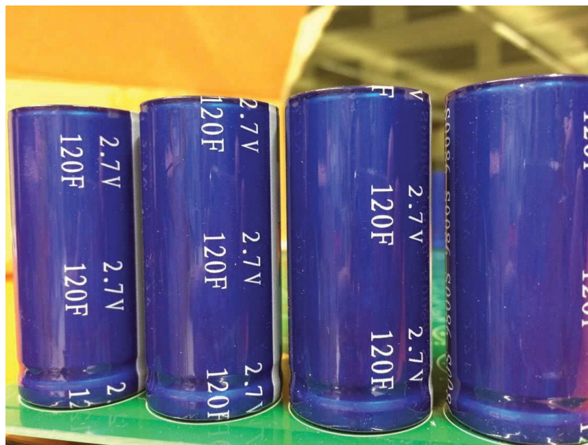
Fig. 3.31 Supercapacitor from Jinzhou Kaimei Power Co.
