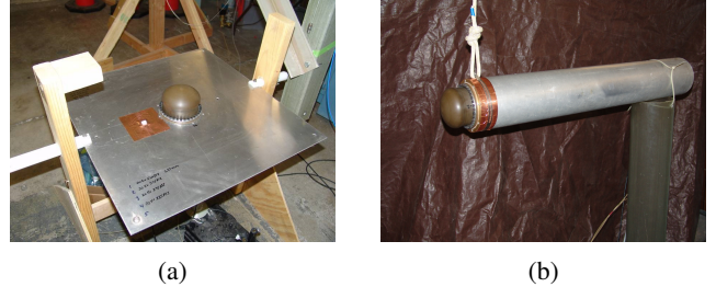
Fig. 3: The spherical EZ antenna in a radome with (a) a 24"x24" ground plane and (b) small ground plane and tube backing
