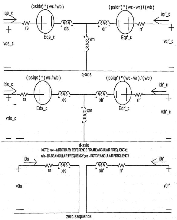
FIG.7.17 EQUIVALENT CIRCUIT OF THREE PHASE I.M. IN ARBITRARY REFERENCE FRAME
