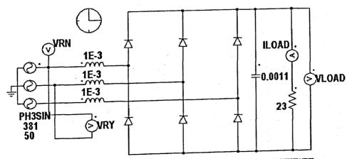
FIG. E.5: THREE PHASE FULL WAVE DIODE BRIDGE RECTIFIER
