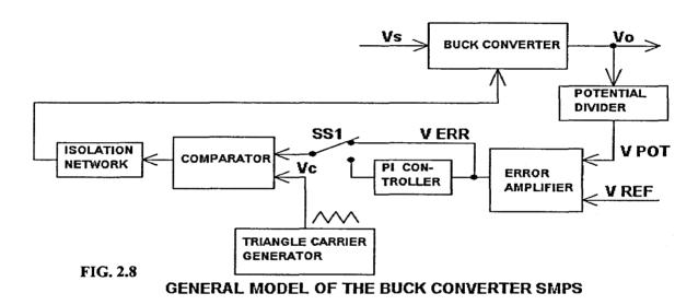
This thesis provides a new interactive system model for a buck converter SMPS suitable for power electronics laboratory applications, a schematic of which is shown in Fig.2.8. Switching function concept is used in developing this model [54-56].
