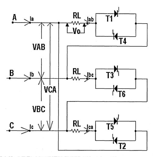
FIG.6.20: DELTA CONNECTED THREE PHASE AC THYRISTOR CONTROLLER
