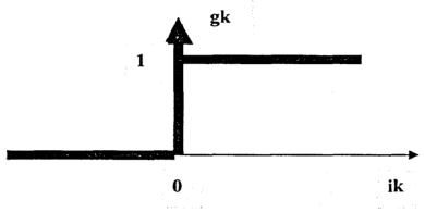
The system model for three phase FWDBR is developed based on reference 61. Heaviside function gk for k = 1,2,3 ... is defined in Fig.3.14. This Heaviside function determines whether the diode is conducting or in the blocking
