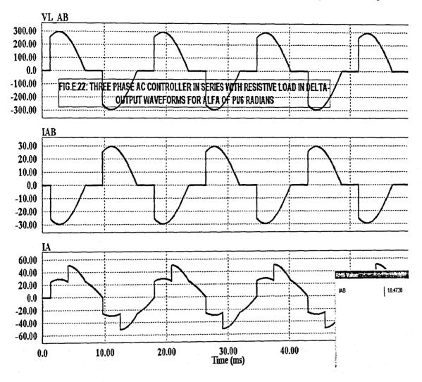
The data for this three phase ac controller shown in Fig.E.21 are taken from Table 6.4 in Section 6.3.2 of Chapter 6. The simulation results of Fig.E.21 for a firing angle of 30 degrees is shown in Fig.E.22, which agrees with the corresponding waveforms shown in Fig.6.24(A), (B) and (C) in Section 6.3.2. The r.m.s. phase current displayed in Fig.E.22 is 18.4728 Amperes which almost agrees with the value in Table 6.5 of Section 6.3.2.
