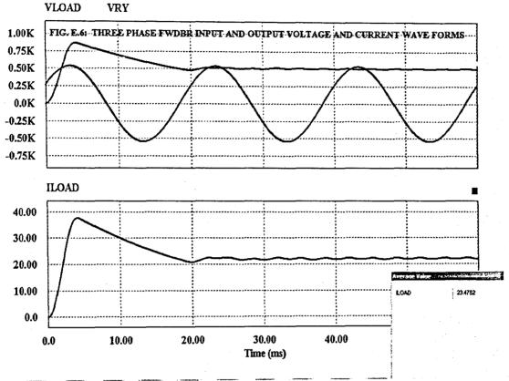
amperes, which closely agree with the corresponding value shown in Table 3.5 of Section 3.4.2. The simulation results in Fig.E.6 also agree with one shown in Fig.3.19 (A), (B) and (C) of Section 3.4.2.
