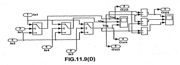
shown in Fig.11.9(A) to (E). Fig.11.9(A) correspond to the dialog box "Three Phase THIPWM Inverter and Triangle Carrier Wave Generator Unit" in Fig.11.8. The various subsystems are: Three Phase THIPWM Generator, Triangle Carrier Wave Generator and Three Phase VSI.
