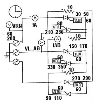
FIG.E.21: THREE PHASE AC CONTROLLER IN SERIES WITH RESISTIVE LOAD IN DELTA
