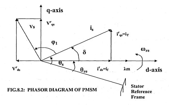
control of PMSM is derived from its dynamic model. Considering the currents as inputs, the three phase currents are given below in equation 8.9.
