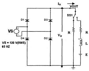
FIG.1: SINGLE PHASE DIODE BRIDGE RECTIFIER
