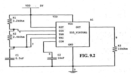
Referring to Fig.9.2, the clock frequency  $f_C$  is given by the formula given in equation 9.1 below:
