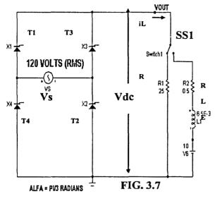
: SINGLE PHASE FULL WAVE SCR BRIDGE RECTIFIER
