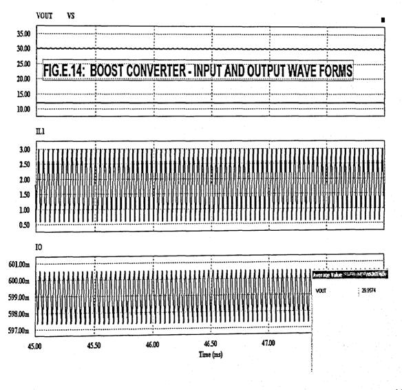
Table 5.4 of Section 5.3.2. The simulation results for Vout, IL1, Io and the displayed output voltage of 29.9574 Volts in Fig.E.14 well agree with the Table 5.5 and Fig.5.12(A) to (D) in Section 5.3.2.
