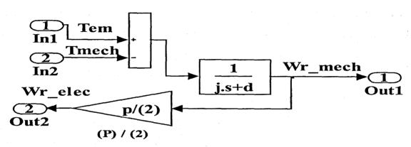
FIG.8.5(I): ROTOR SPEED CALCULATOR
