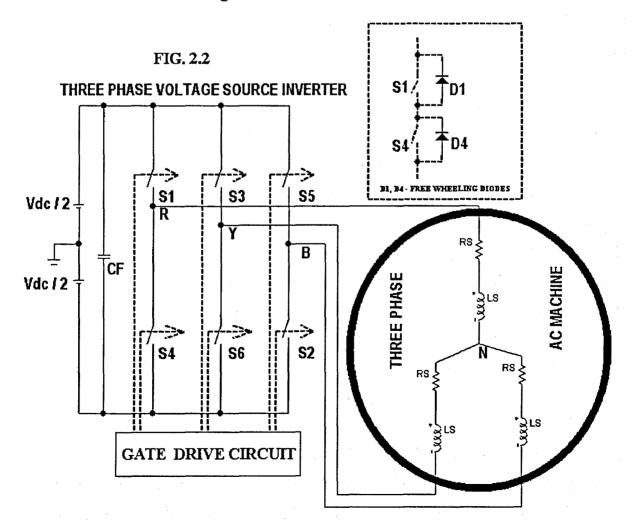
This thesis provides system modelling of three phase 180 degree and 120 degree mode inverter, a general schematic of which is shown in Fig.2.2. User interface is provided where data relating to the particular dc to ac converter can be entered. The models can be copied to various future applications as data entered by the user can be changed without changing the inner details of the model.
