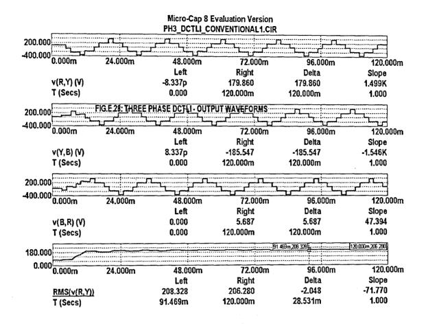
The simulation results are shown in Fig.E.28 for the three phase DCTLI. The r.m.s. value of the line to line voltage Vry indicated in Fig.E.28 is 208 Volts, where as the corresponding value indicated by simulation of the model in Fig.12.5(A) in Section 12.2.2, is 220 Volts..
