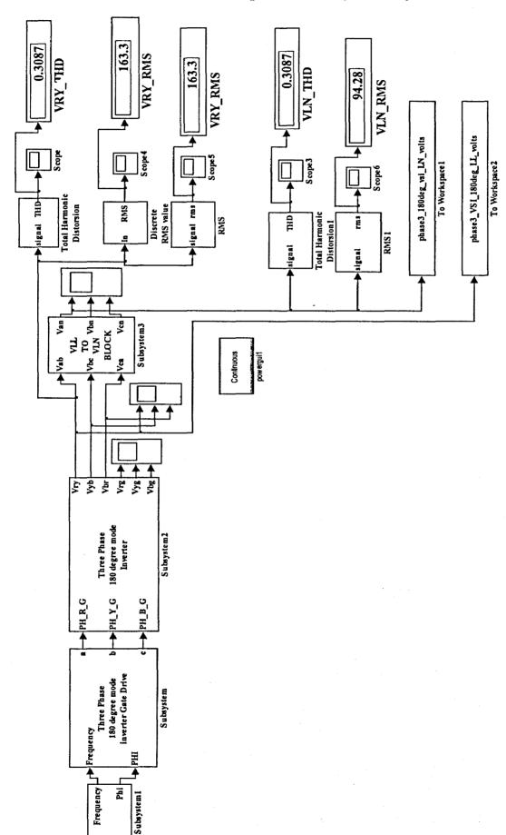
FIG.4.3 MODEL OF A THREE PHASE 180 DEGREE MODE INVERTER
