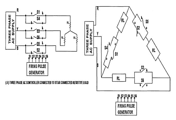
(B) THREE PHASE AC CONTROLLER IN SERIES WITH DELTA CONNECTED RESISTIVE LOAD
