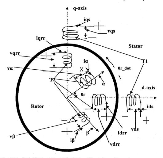
Fig.7.1: Two axis representation of three phase IM
