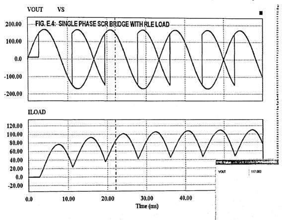
Fig.E.4.for a firing angle  $\alpha$  of  $\pi$  /3 radians. The displayed value of r.m.s. dc output voltage is 117.083 volts, which closely agree with the value in Table 3.4 of Section 3.3.2. The wave forms in Fig.E.4 agree with the Fig.3.12(A), (B) and (C) of Section 3.3.2.
