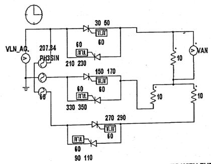
FIG.E.19: THREE PHASE AC CONTROLLER IN SERIES WITH THE LINES WITH STAR CONNECTED RESISTIVE LOAD
