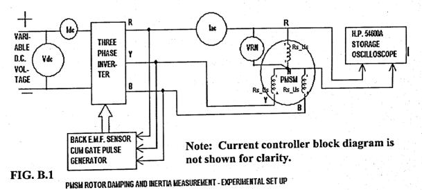
The dc link voltage is initially set to 40 volts. The machine is run on NO LOAD. The initial reading of Vdc, Idc, C.R.O. back e.m.f. period(i.e. initial rotor speed) are noted. The dc input to inverter is switched OFF. The time to fall to various rotor speeds are
