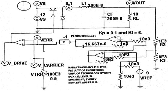
Fig. 10.1(B) BUCK CONVERTER SMPS WITH PI CONTROLLER
