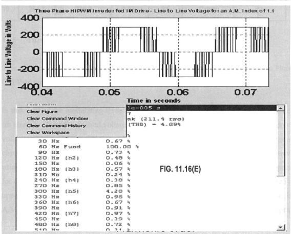
Chapter 11: Modelling of A Three Phase PWM Inverter fed I.M. Drive TABLE 11.3: Line to Line voltage and stator current of Three Phase HIPWM Inverter fed I.M. Drive for an F.M. Index of 33.33
