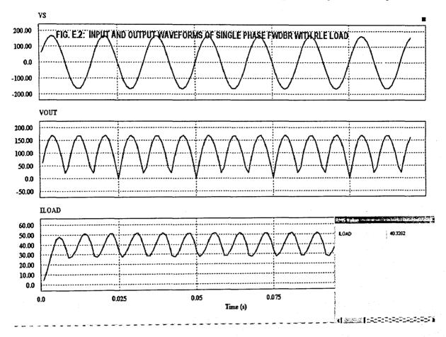
As can be seen from the display of Fig.E.2, it is seen that the rms value of load current is 40.3262 amperes. The results agree with Table 3.2 and Fig.3.6 (A), (B) and (C) of section 3.2.2.
