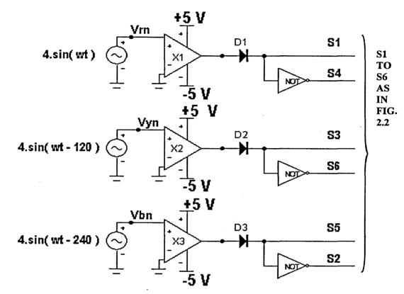
THREE PHASE 180 DEGREE MODE INVERTER GATE DRIVE
