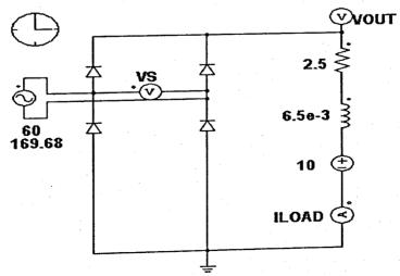
FIG.E.1: SINGLE PHASE FULL WAVE DIODE BRIDGE RECTIFIER
