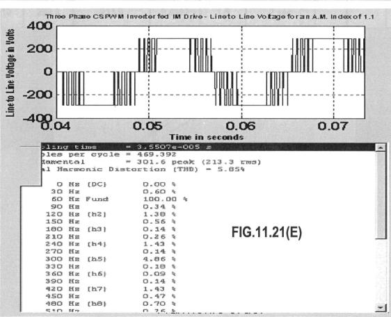
Chapter 11: Modelling of A Three Phase PWM Inverter fed I.M. Drive TABLE 11.4: Line to Line voltage and stator current of Three Phase CSPWM Inverter fed I.M. Drive for an F.M. Index of 33.33.
