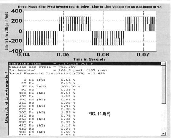
Chapter 11: Modelling of A Three Phase PWM Inverter fed I.M. Drive TABLE 11.1: Line to Line voltage and stator current of Three Phase Sine PWM
