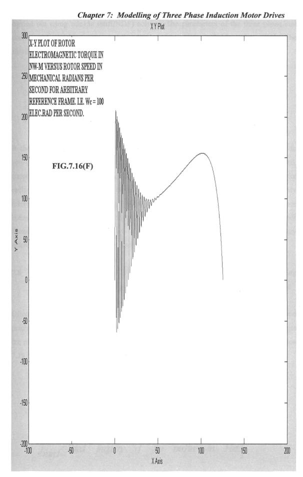
Chapter 7: Modelling of Three Phase Induction Motor Drives carried out using ode15s (stiff/NDF) solver. The parameters of the three phase star connected squirrel cage IM used for simulation are given in Table 1 above [10]. The simulation was carried out in the following reference frames:
