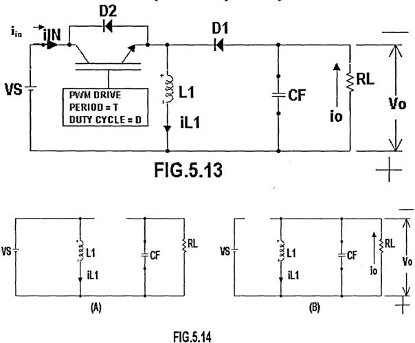
ent is continuous or always greater than zero. Noting that the change in inductor current during the ON time and OFF time are equal or the average inductor current over one switching cycle is zero, the following equations can be derived.
