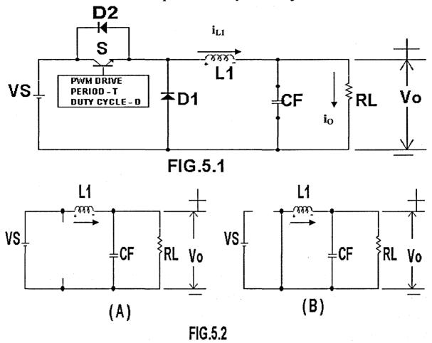
equivalent circuit of Fig.5.1 when the switch is ON from 0 to DT seconds and OFF from DT to T seconds respectively. This analysis assumes CCM, i.e the inductor current ent is continuous or always greater than zero. Noting that the change in inductor current during the ON time and OFF time are equal or the average inductor current over one switching cycle is zero, the following equation can be derived.
