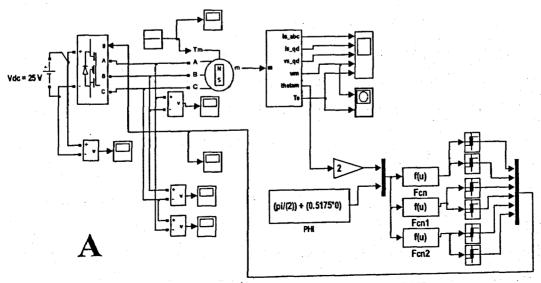
FIG.E.25: SIX STEP 180 DEGREE MODE INVERTER FED PMSM DRIVE
