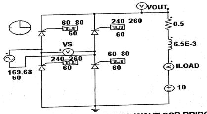
FIG.E.3: SINGLE PHASE FULL WAVE SCR BRIDGE
