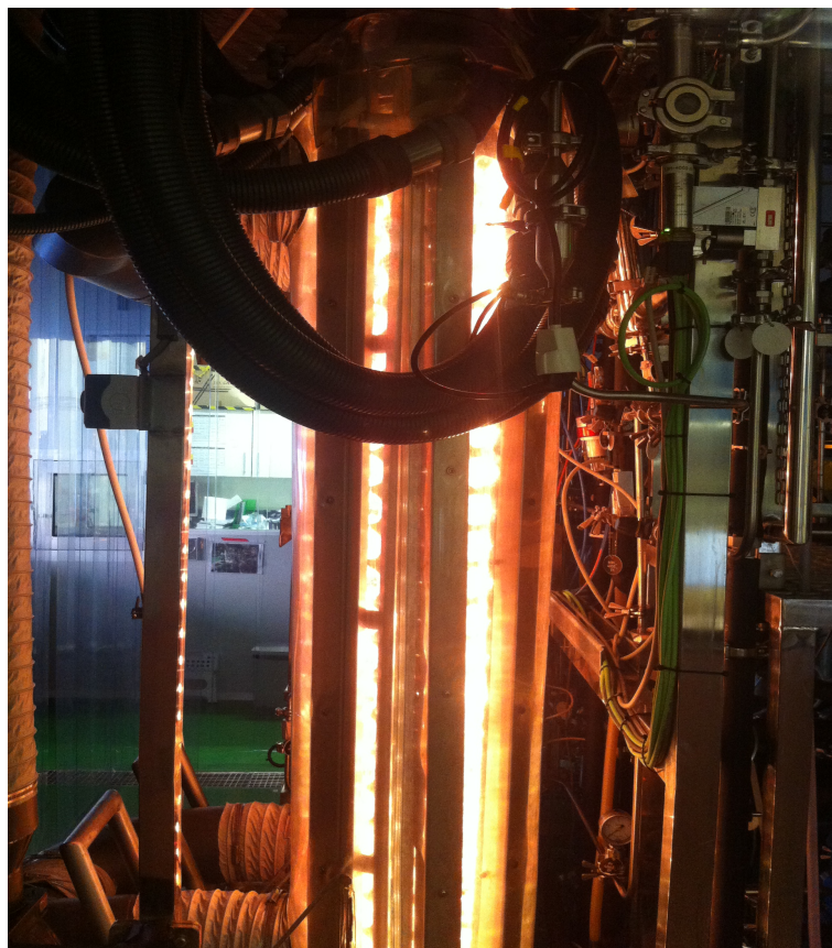
Picture 3- The photosynthesis compartment (IVa). Water and carbon-dioxide inputs are transformed by cyanobacteria of the genus Arthrospira ('spirulina') into oxygen and edible biomass. Photographed by authors (25 th November 2015)
