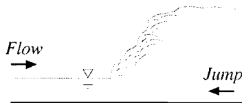
Figure 7: Sketch of the relative motion of the hydraulic jump and flow
