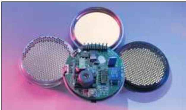
Figure 6: The SensComp series 600 SmartSensor (rear view showing the integrated interface board at centre)
