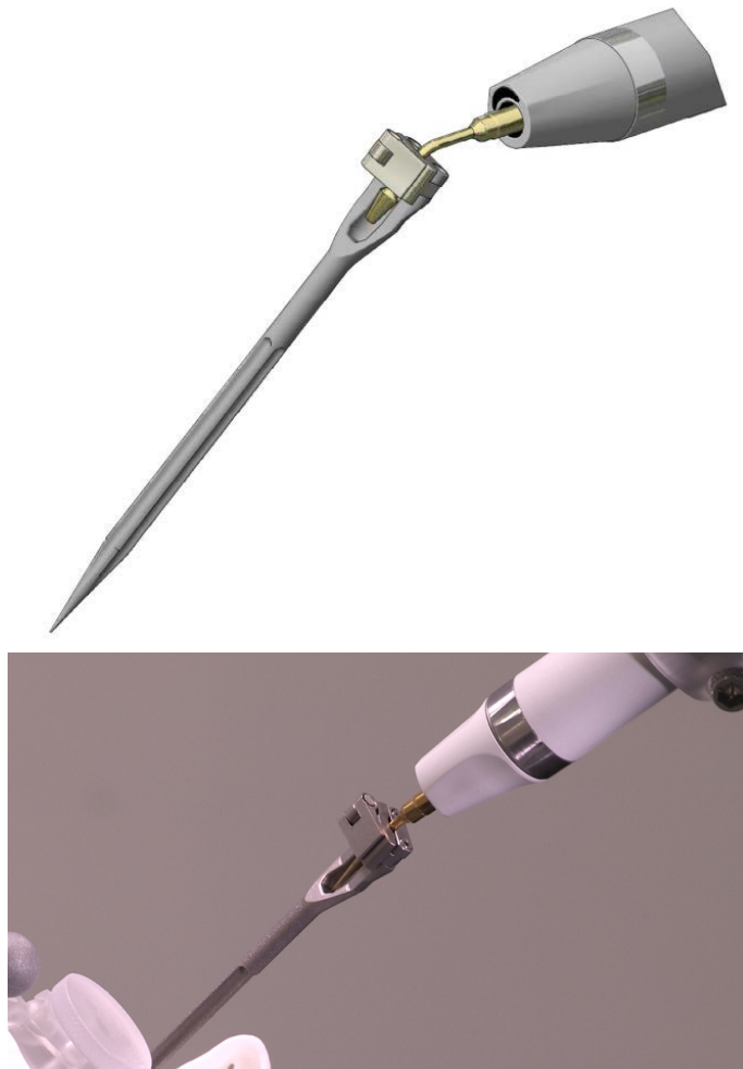
Fig. 6.5 Piezoelectric handpiece long probe calibration, CAD model (top) and physical prototype (bottom): the top clamp holds the terminal cutting part of the piezoelectric tip in axis with the rest of the calibration device, ensuring stability during the pivoting action.
