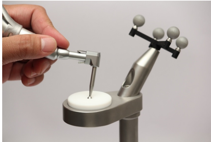
Fig. 6.12 Original design for a calibrating instrument: short and long straight tips are used to pivot around a point fixed in three dimensions with respect to the patient's optical reference tool.
