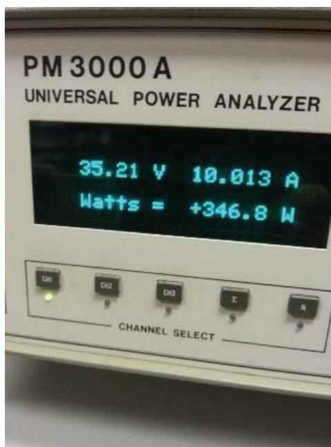
Fig. 5.29. The voltage, current and power to the load.
