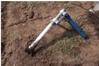
Figure 8.5 The cable ploughing and irrigating prototype. Note - in order to prevent breakage on large survey jobs where obstacles would be encountered, a spring would need to be incorporated into this design. A press wheel also needs to be added to press down soil clods onto the cable.
