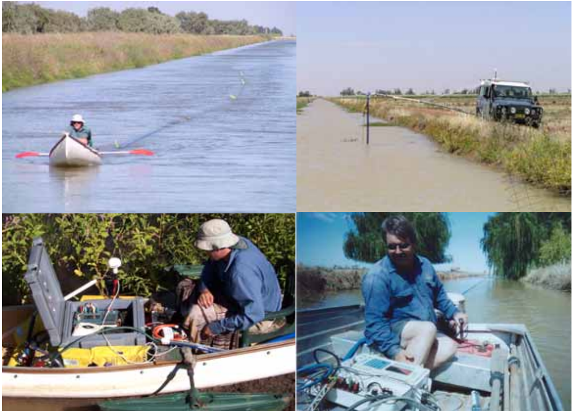
Figure 7.3 Equipment for towed geo-electric surveying from surface water bodies. Small watercraft such as canoes with outboard motors are appropriate in canals which typically contain numerous obstacles over which the craft must be lifted either by hand or with a small crane. In canals with lots of weed, which quickly stops outboard motors, a boom extending from a 4wd is most appropriate for towing arrays. Electronics suitable for operating the arrays is produced by Lund university combined with ABEM – Terraohm RIP924, Iris Instruments – Syscal Pro (lower left), Zonge – GDP32 (lower right) and AGI – Supersting R8 Marine.
