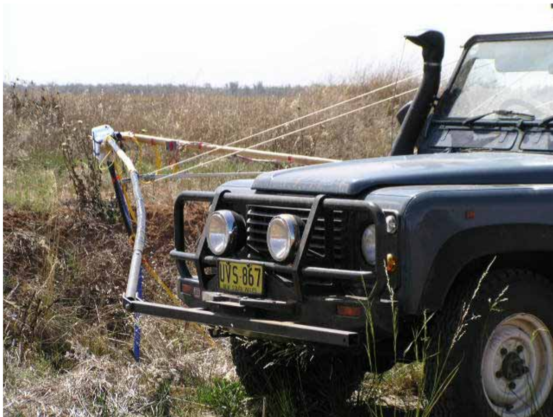
Figure A2-6 Using a boom towed array, farm canals, furrows and rice bays with less than 20mm of water in the bottom of them could be surveyed as shown. Data from such canals had to be filtered with a low current filter due to the current electrodes coming out of the intermittent water at some locations.
