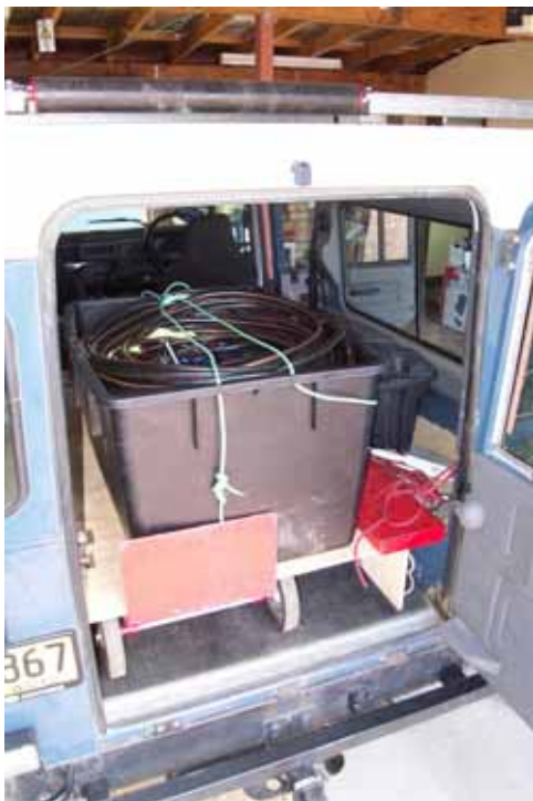
Figure 7.2 A 144m geo-electric array deflated and packed for land transport. The last 64m of the array are seen at the top of the box (single wire in garden hose). The rest of the array consists of heavy gauge multicore cable glued to layflat hose.
