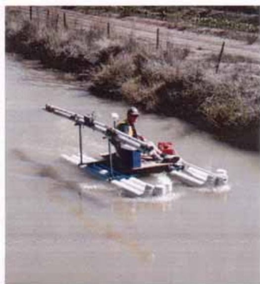
Figure A7-9 EM-31 surveying of an irrigation canal using a lightweight non-metallic water craft. (from Harding, 2002).
