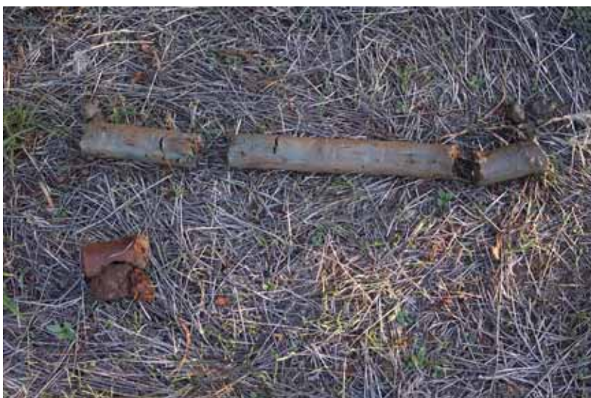
Figure A7-2 Yabby pump samples of both soft permeable waterlogged clay core (grey) and hard impermeable clay core (red). Note the different penetration depths attained.
