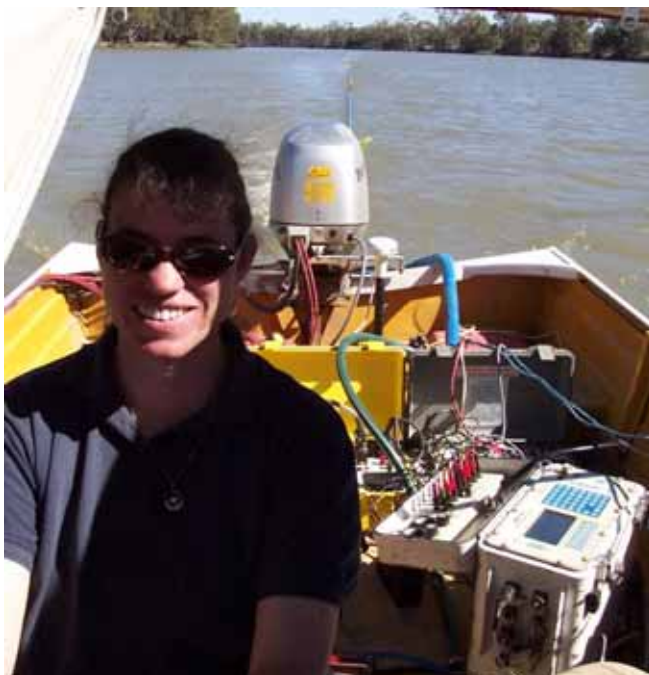
Figure A2-1 A 144m array being towed by a 14' boat with 40hp 4 stroke motor on the Murray River near Mildura.
