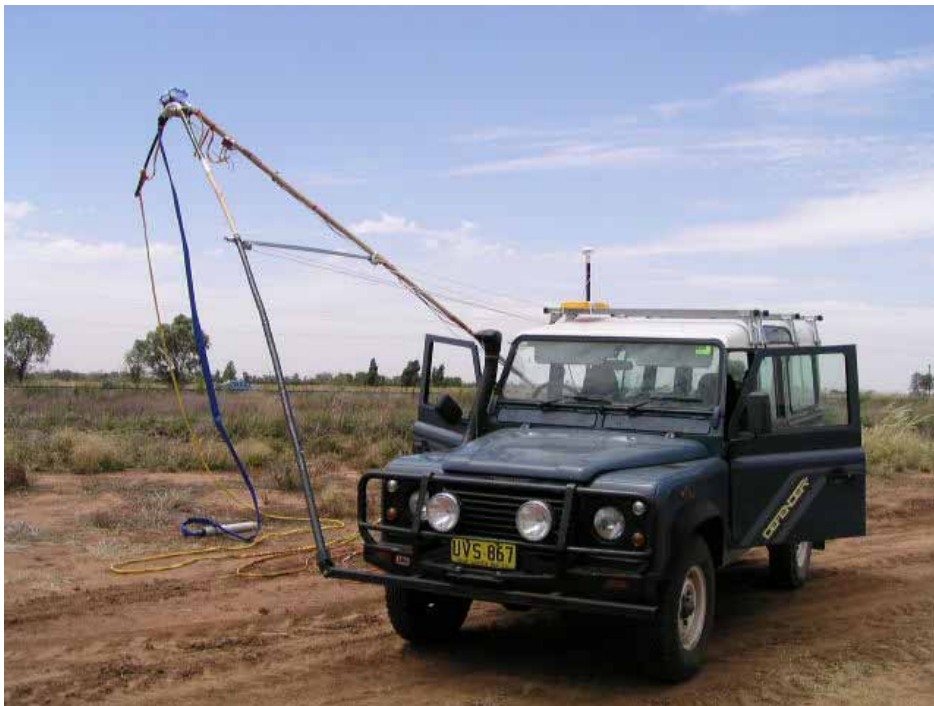
Figure A2-5 The boom partially raised in preparation for high speed travel. The blue tube towed a pressure sensor which, on this survey was not incorporated into the array due to short term rental.
