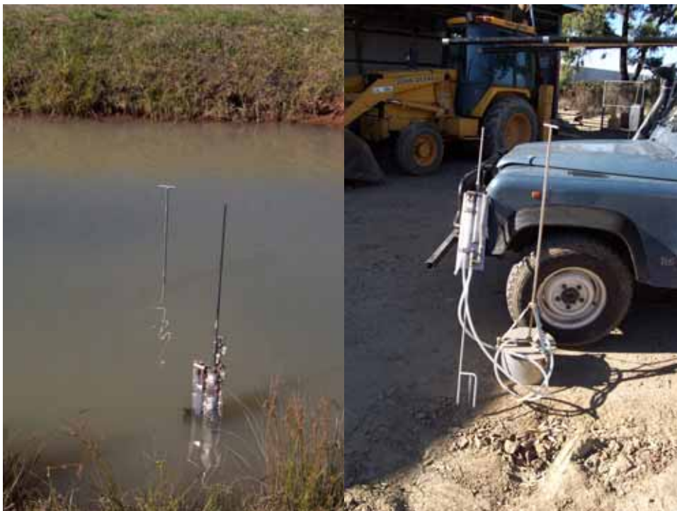
Figure A7-5 An Idaho seepage meter.
