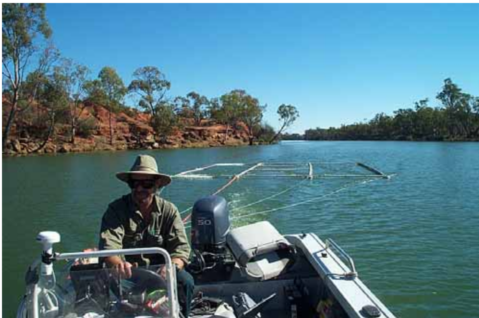
Figure 2.5 A floating transient electromagnetic device (Zonge NanoTEM) on the Darling Anabranch
