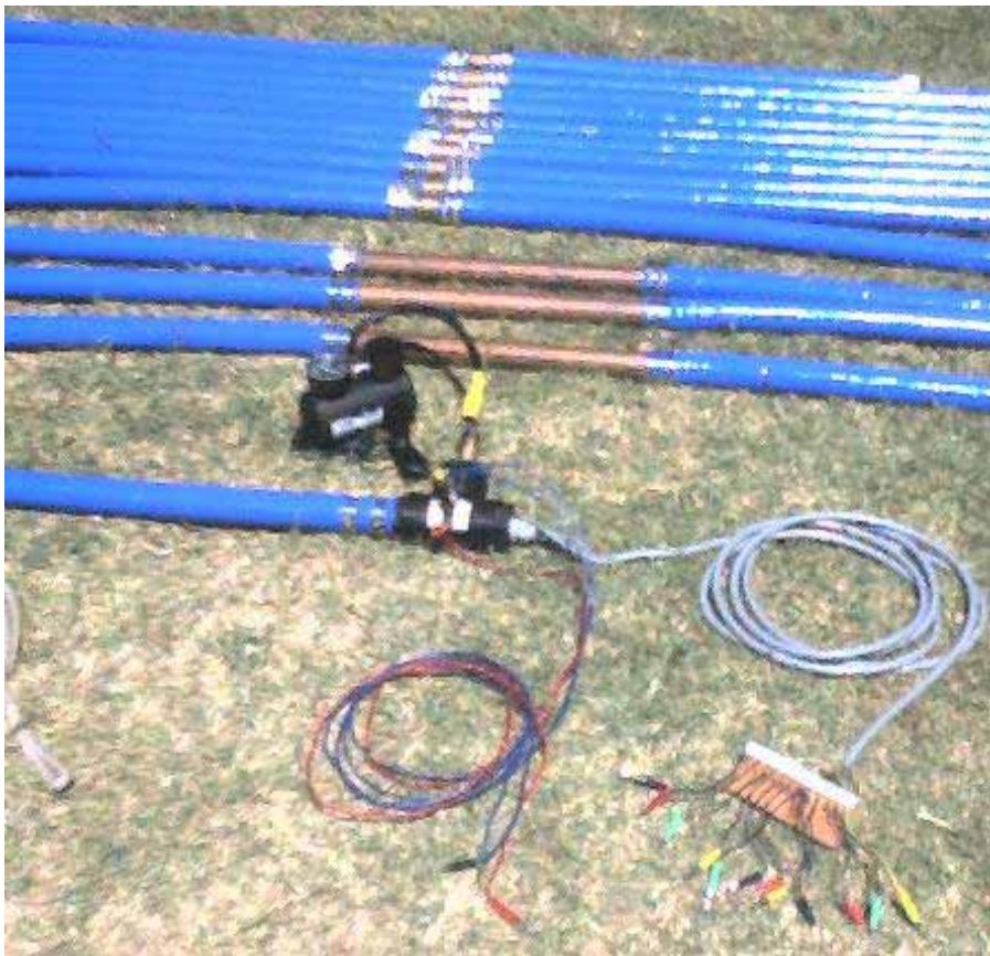
Figure A1-3 An old rejected design of geo-electric array in which all wires and a strain bearing cable are inside the float tube.
