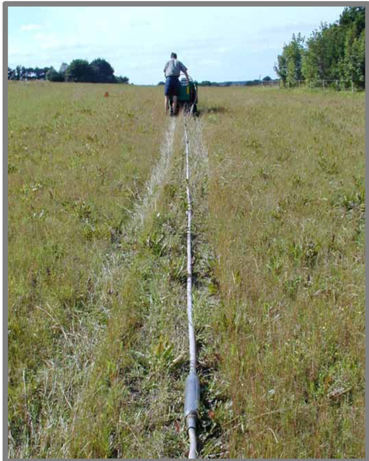
Figure 8.4 The Pulled Array Continuous Electric Sounding (PACES) system imaging a depth interval from 0.5 to 20m in Denmark.
