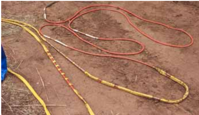
Figure 7.1 An early prototype submersible 20m geo-electric array (with 15m yellow leader).
