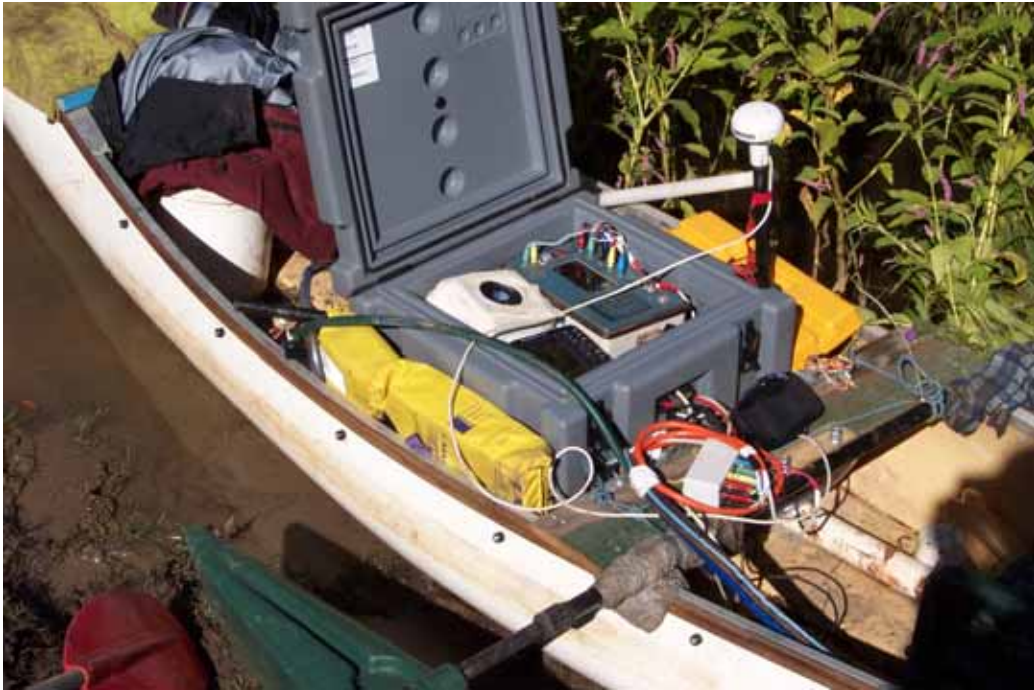
Figure 7.8 The EC data acquisition subsystem – Iris Syscal Pro (supplied by Geoforce) incorporated into a sealable water cooled box with GPS and sonar equipment.
