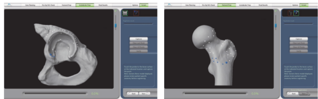
Fig. 1. Registration pattern for pelvis and femur in MAKO [10]. The dots show the bony landmarks to be accurately verified and acquired by the probe for registration.
