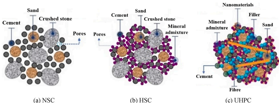
Fig. 1. Material compositions of NSC, HSC and UHPC [2].
