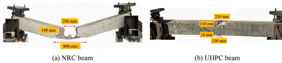
Fig. 24. Comparison of the response of 2440 mm × 250 mm × 125 mm simply-supported NRC and UHPC beams with GFRP rebars to free-air burst at Z = 0.22 \text{ m/kg}^{1/3} [83].
