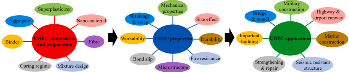
Fig. 4. Development of UHPC: from material composition and sample preparation to material properties and applications.
