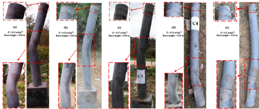
Fig. 30. Bottom fixed UHPC-FST columns against near-field explosions under air burst environment [132].
