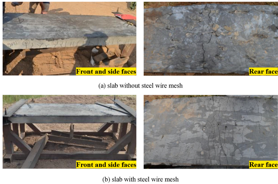
Fig. 27. Comparison of 2000 mm × 800 mm × 120 mm partially fixed one-way high strength self-compacting concrete slabs with or without steel wire mesh at Z = 0.66 \text{ m/kg}^{1/3} under free-air burst environment [70].
