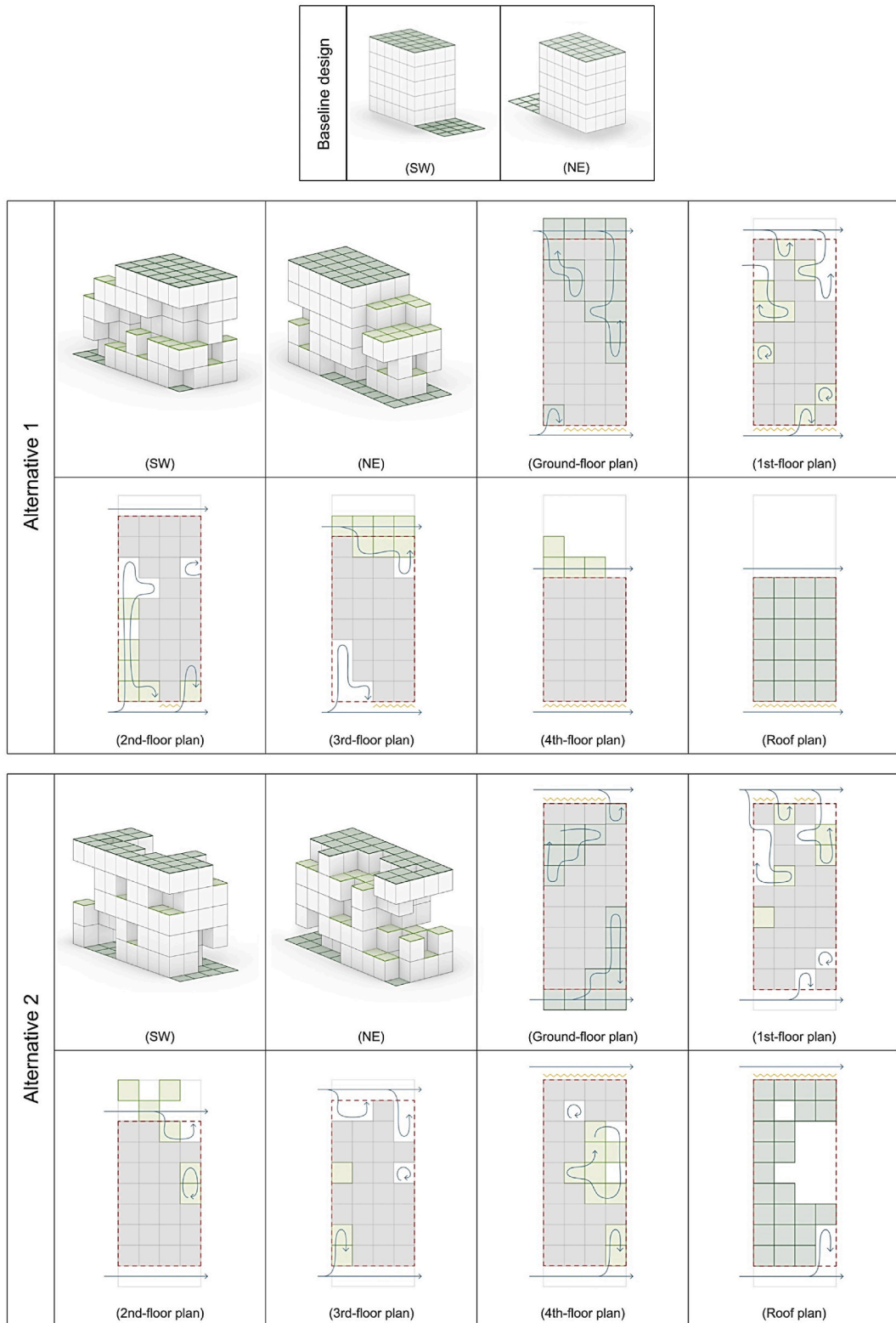
Fig. 12. Comparison of the baseline Building Mass in Tehran with Four Optimized Alternatives: Visualization of the Pareto front in objective space, with illustrative design images. The multi-objective optimization results are plotted (perhaps in a 2D or 3D graph within Octopus plugin), and three representative solutions are highlighted: (a) a solution from the extreme end favoring maximum solar (lots of terraces); (b) a solution favoring compactness (minimal terraces, similar to baseline performance); (c) a balanced solution (Pareto-optimal).
