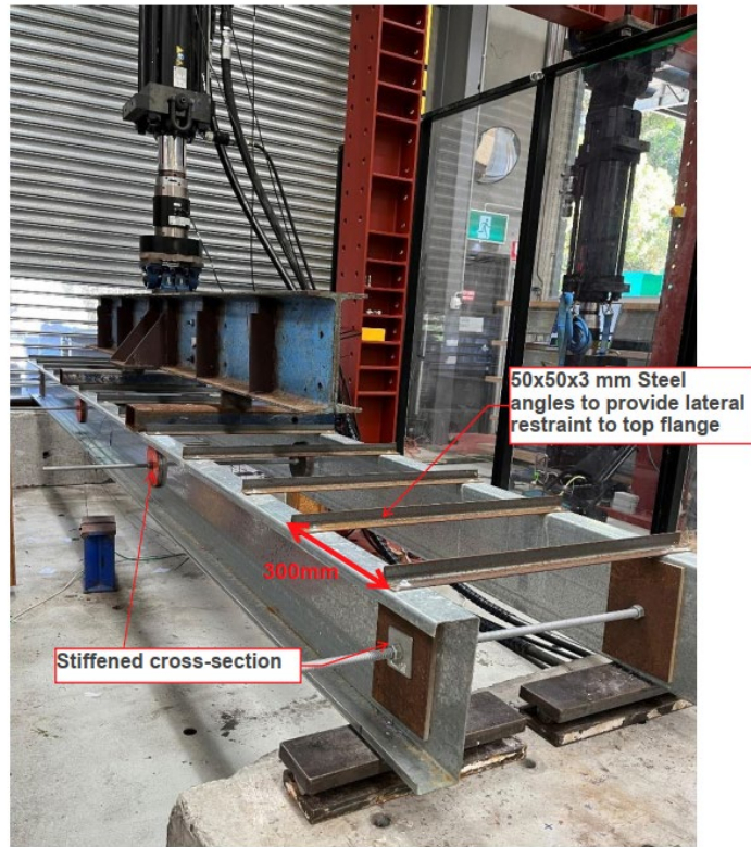
Fig. 3. Overall test layout of bare CFS beam tests
