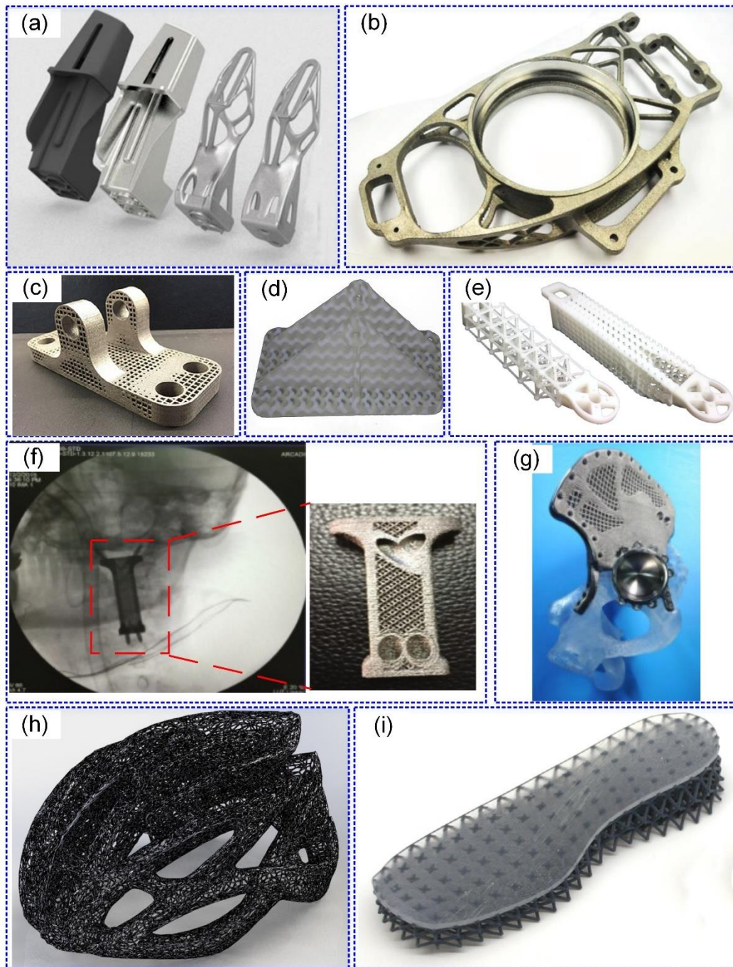
1945 Figure 33. Examples of applications. Automotive engineering: (a) roof brackets for BMW i8 Roadster [36], (b) rear upright of car suspension [37]. Aerospace engineering: (c) metal aero bracket [38], (d) jet engine bracket with interpenetrating phase composite [367], (e) quadcopter's arm [787]. Load-bearing tissue scaffolds and implants: (f) cervical vertebral fusion cage [792], (g) hemi-pelvic [799]. Other applications: (h) bicycle helmets [44]; (i) shoe sole [45]. 1950
