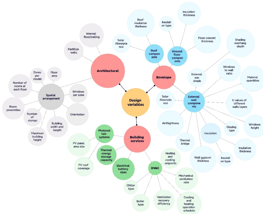
Figure 4. Design variables divided into three clusters of architectural, building services, and envelope. Source: The authors
