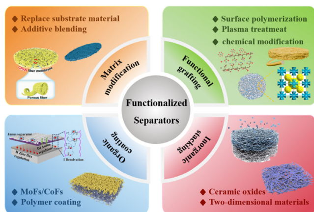
FIGURE 4 | Schematic diagram of engineering strategies of separators for AZIBs.
