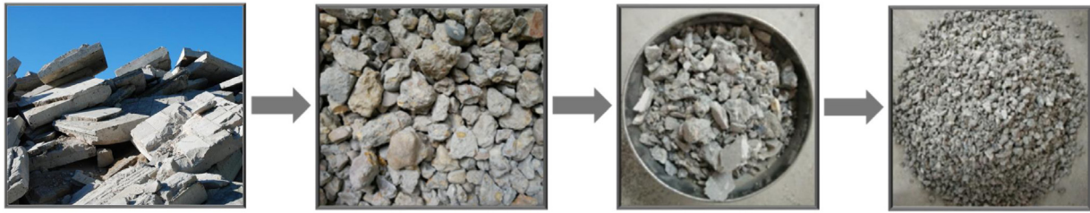
Fig. 1 – Resource and manufacturing of recycled aggregates.
