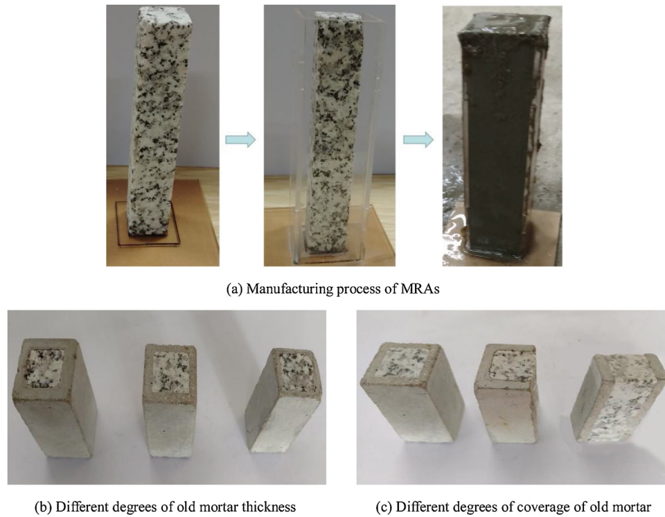
Fig. 2 – MRA prepared with different thickness and coverage of old mortar.
