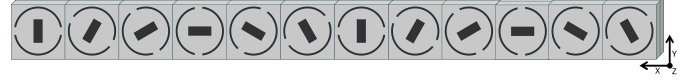
Fig. 8. Three-dimensional view of the 1 \times 12 supercell array, composed of optimized PR unit cells with an incremental 30^\circ rotation between adjacent elements along the x-axis.
