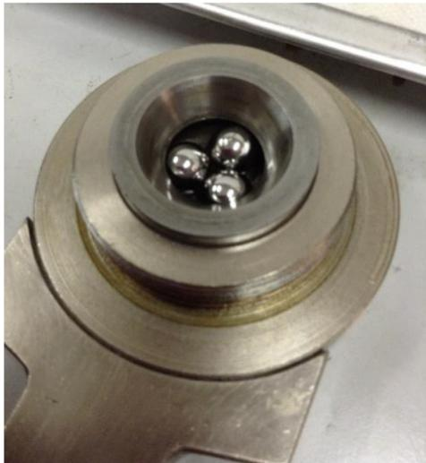
Fig. 1. Four ball tribo-tester cup.
