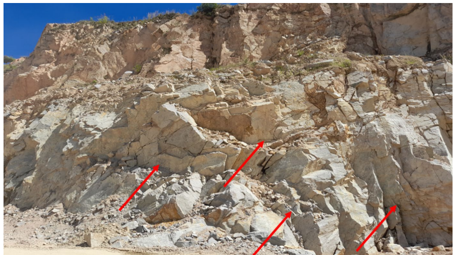
Fig. 4 Blocky rock mass with cubical blocks defined by rough, slightly weathered joints. It is challenging to blast smooth faces because of ragged excavation surfaces caused by small wedge or block failures
