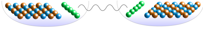
FIG. 1. A collection of trapped ions in two separate elementary logical units (ELUs). Some of the ions in each trap are used to encode a logical surface code qubit while other communication ions collect and refine entanglement to be used for a two-qubit lattice surgery operation.
