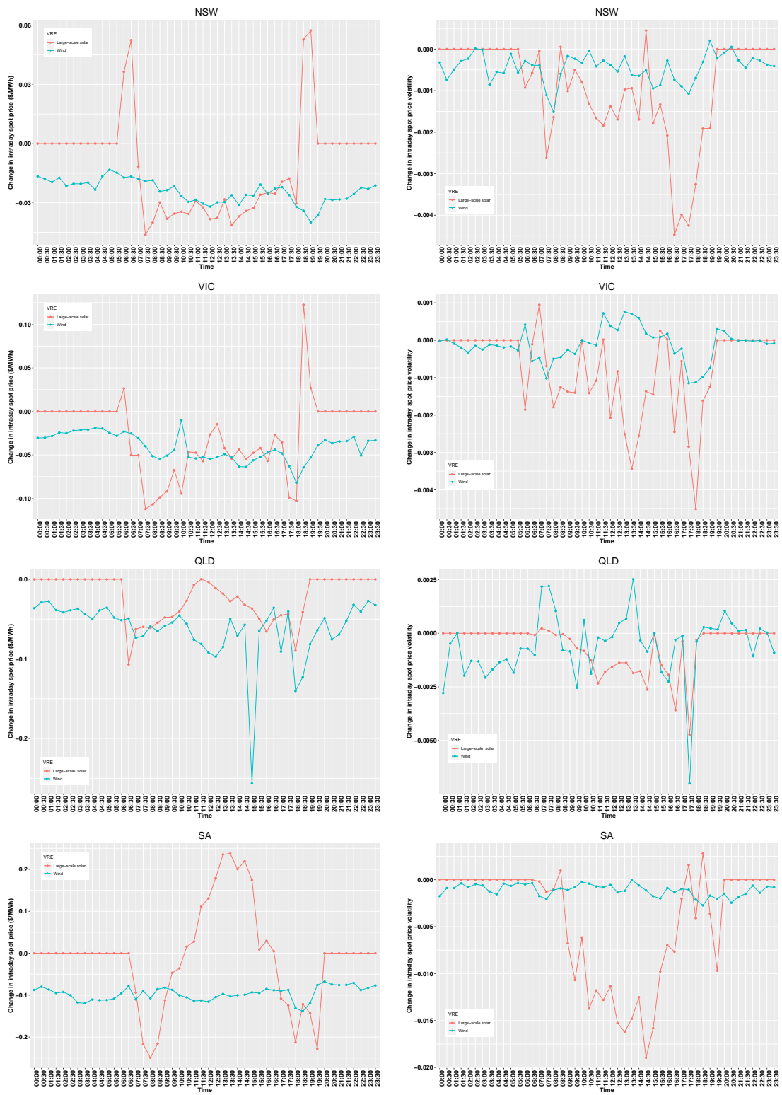
Figure 7: Change in spot electricity prices (left panels) and volatility (right panels) per MWh increase in large-scale solar and wind generation for NSW, SA, VIC, and QLD
